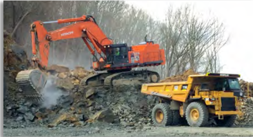
Hitachi 1200 loading CAT 773 with shot rock Seg. 2b/3a
